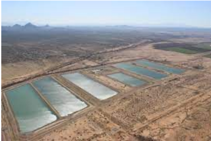
Colorado River water is conveyed via CAP to the Avra Valley recharge facilities for infiltration.
