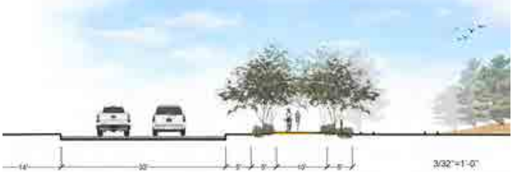
(A) two-way multi-use trail that is tightly aligned to the Arizona Eastern Railway tracks. This segment has delineated wooden frames and accent plants to buffer from the train.
