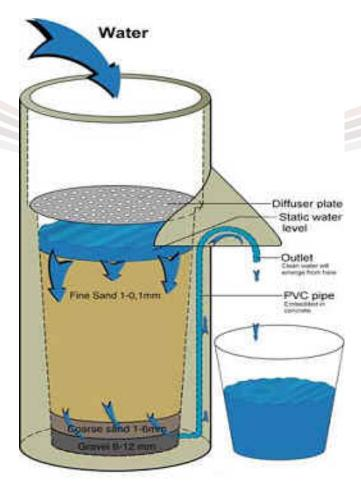
A slow sand filter remove the smallest particles. A slow and constant flow of water through the filter described above leads to **biological activity** as the top layer of sand traps micro-organisms (e.g. bacteria). *"bio-film* builds up on top of the sand." RSS Quality
