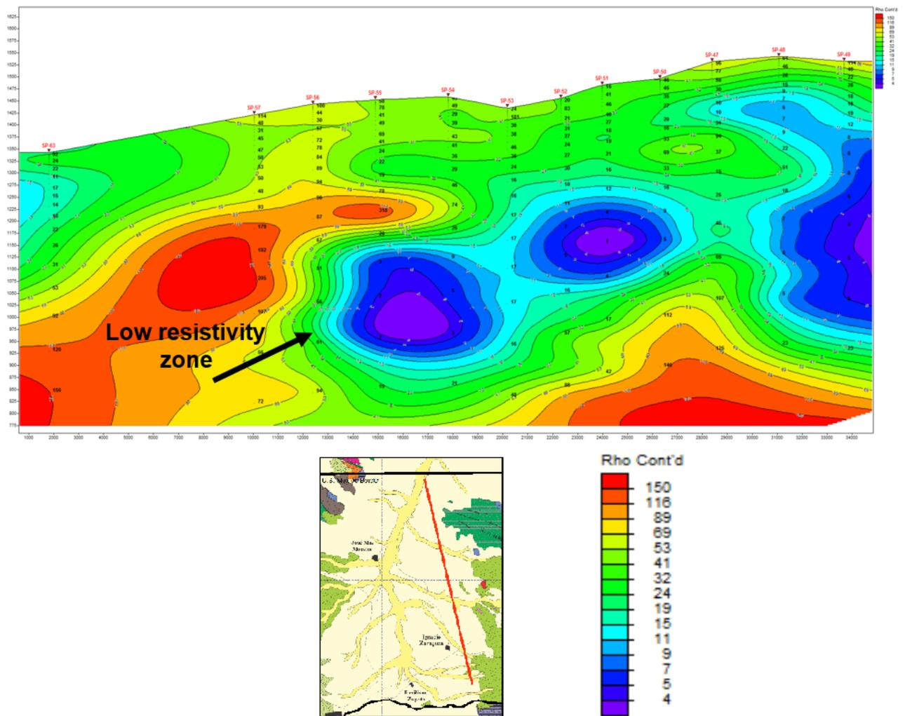
**Figure 5.1** North-South Resistivity Profile (TEM) developed on the Eastern Boundary of the Mexican Side of the Binational San Pedro Basin, showing the low resistivity zone (dark-blue and purple contours) that could be associated with faulting of the basement. Location of the profile is indicated by the red line on in the geologic map in the lower portion of the figure (For detailed geology see Figure 4.1). Distances on resistivity profile and map are in meters.
