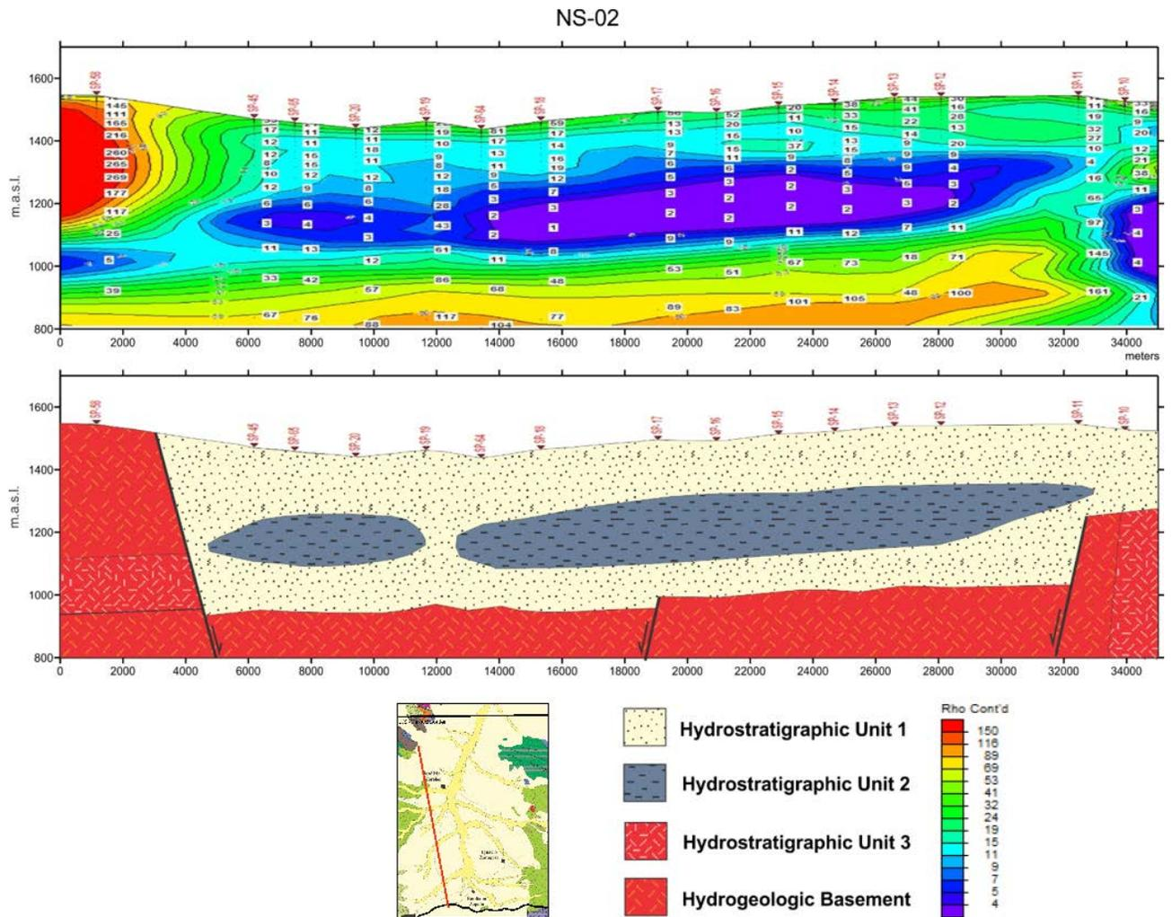
**Figure 5.2 Proposed Distribution of Hydrostratigraphic Units Based on Resistivity (TEM) Profiles (and other information) carried out on the Eastern Boundary of the Mexican Side of the Binational San Pedro Basin. Location of the profile is indicated by the red line on in the geologic map in the lower portion of the figure (For detailed geology see Figure 4.1). Distances on resistivity profile and map are in meters.**
