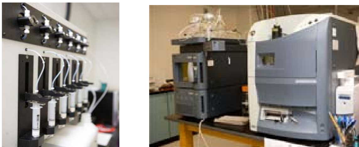
Figure 3. Autotrace solid phase extraction workstation (left) and liquid chromatography tandem mass spectrometer (right). Instruments are located at the UA's Arizona Laboratory for Emerging Contaminants.
