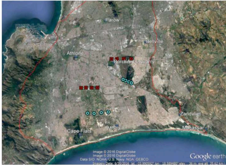
Figure 5-1 Hypothetical abstraction (blue circle) and injection (red square) sites with WWTW shown in white text, groundwater model boundary shown as red line.
