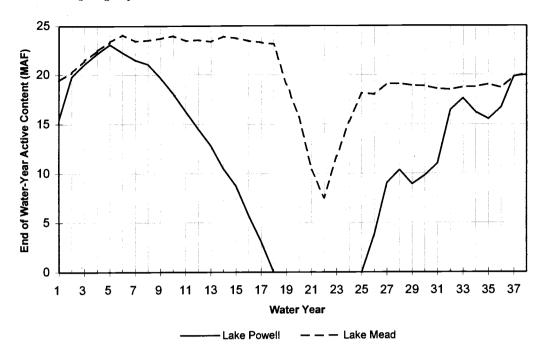
Figure 3. Lake Powell and Lake Mead End of Water-Year Active Contents Under the Baseline, with SSD Inflow Hydrology.
