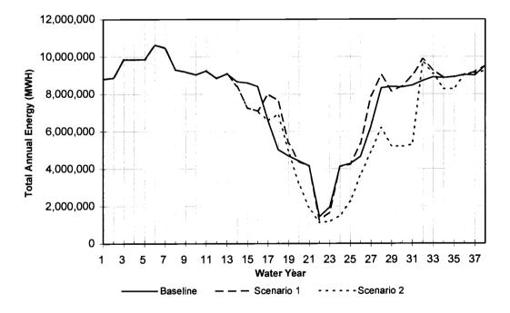
Figure 7. Total Annual System Energy Generated Under the Baseline, Scenario 1, and Scenario 2, with SSD Inflow Hydrology.
