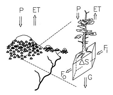
Figure 1. Sketch Illustrating Water-Balance Components Important in Tree-Ring Reconstruction of River Flow. Variables are precipitation (P), evapotranspiration (ET), surface and subsurface inflow and outflow  $(F_i$  and  $F_o)$ , percolation to ground water (G), and change in soil moisture  $(\Delta S)$ .
