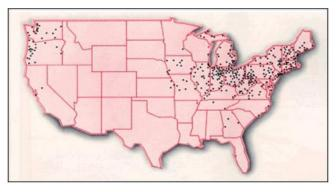
Figure 4: Locations in the US with combined sewers<sup>14</sup>
