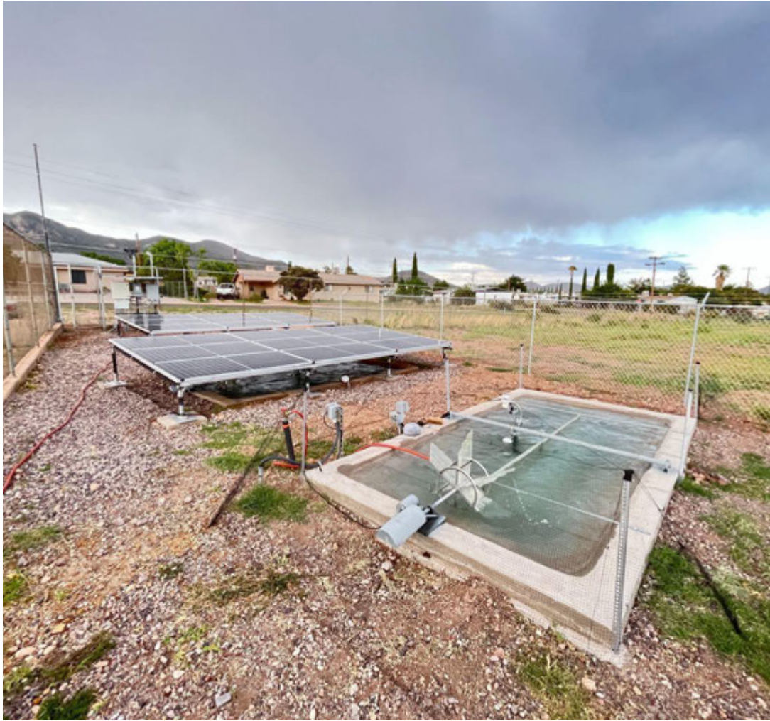
The Bisbee Science Lab Prototype; Two sets of solar panels, one over dry land and another over a pond, with an open pond in the forefront of the image.
