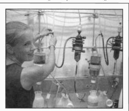
MS student Bridgette Howard samples her two permeable reactive barrier columns for treating acid mine drainage containing 25 mg/l copper.
