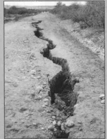
The above may look like an earth fissure caused by groundwater pumping but is, in fact, a desiccation crack running down a Graham County road. Photo: Raymond C Harris.
