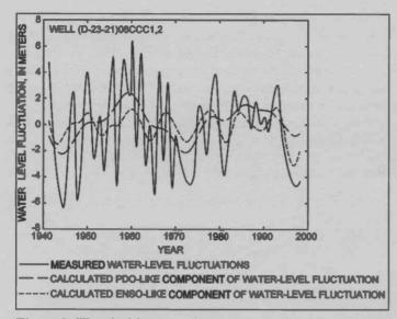
Figure 2. Water-level fluctuations from a well in the Upper San Pedro Basin in southeastern Arizona and two calculated patterns of periodic behavior used in the inverse process.
