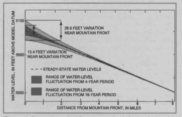
Figure 3. Range of water-level fluctuations of the idealized model for cyclical recharge rates of 4- and 16-year periods.
