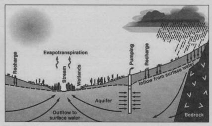
Figure 1. Cross-section of an idealized aquifer in the Southwestern United States. Ground water flows from recharge areas near mountain fronts to discharge areas near streams and wetlands.
