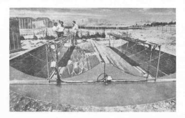
Figure 3. A floating photovoltaic concentrator converts solar radiation to electricity used to operate water-moving pumps.
