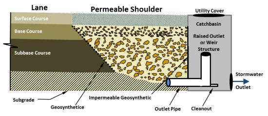
Figure 9.4. Typical underdrain outlet detail (urban section).
