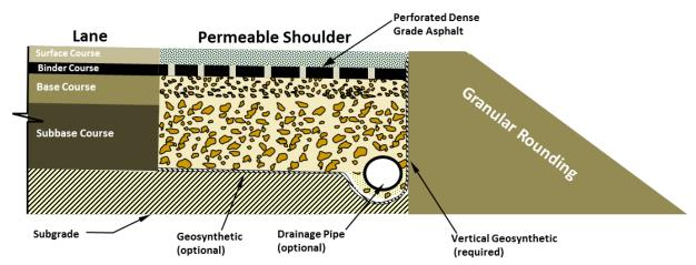
Figure 6.2. Conceptual strengthened permeable shoulder.
