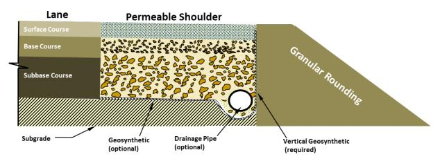
Figure 6.1. Basic permeable shoulder configuration.
