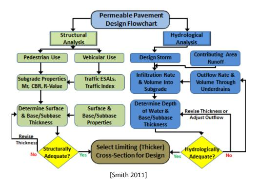
Figure 5.1. Structural and hydrological design flowchart.
