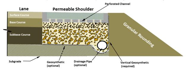
Figure 6.3. Conceptual channeled permeable shoulder.
