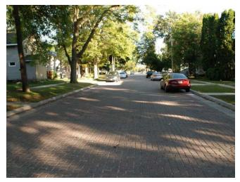
Figure 3.5. Permeable interlocking concrete pavement.
