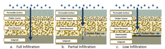
Figure 3.2. Permeable pavement infiltration types.
