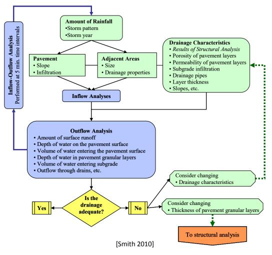
Figure 5.2. Hydrological design process.
