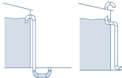
Figure 6 Examples of tank overflow outlets
