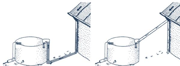
Figure 1 Examples of wet (left) and dry (right) conveyance systems
