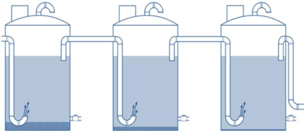
Figure 2 Multiple tanks connected in series
