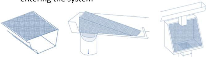
Figure 3 Common gutter and downspout screens
