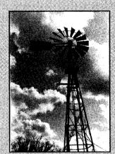
The windmill is a low-tech device for bringing groundwater to the surface.
