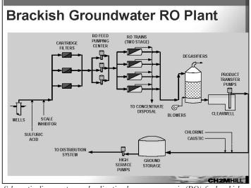
Schematic diagram traces desalination by reverse osmosis (RO) for brackish groundwater. Source: CH2MHill.
