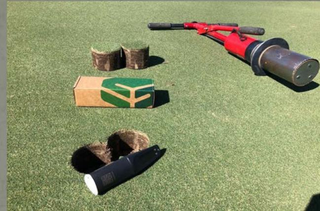
Above: Pogo Moisture Meter, Below: Spectrum Moisture Meter.
