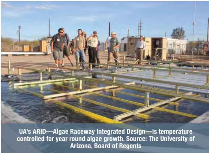
UA's ARID—Algae Raceway Integrated Design—is temperature controlled for year round algae growth. Source: The University of Arizona, Board of Regents
