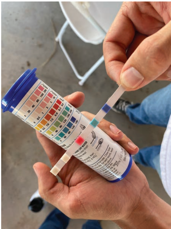
Figure 7.1 Home water-testing kits typically rely on a color change on a test strip to determine the concentration of a contaminant. Source: Lynn Carroll
