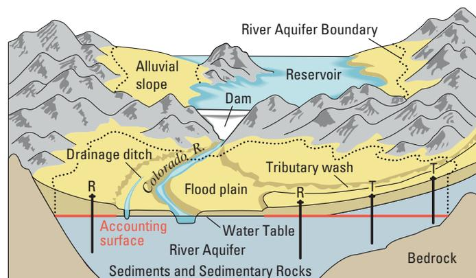
**Figure 1.** Schematic diagram showing the river aquifer and accounting surface. Wells labeled "R" have a static water-level elevation equal to or below the accounting surface and are presumed to yield water that will be replaced by water from the river. Wells labeled "T" have a static water-level elevation above the accounting surface and are presumed to yield water that will be replaced by water from precipitation and inflow from tributary valleys (Modified from Wilson and Owen-Joyce, 1994).
