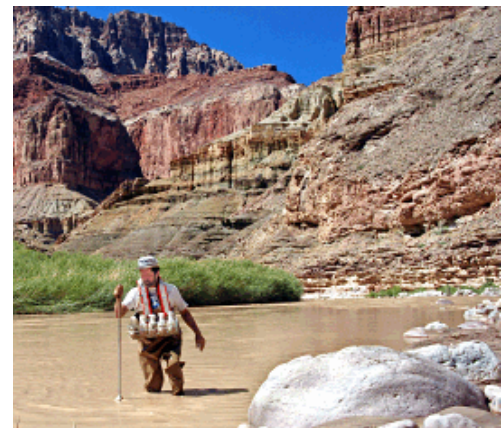
FIGURE 2 - SAMPLING IN-STREAM SUSPENDED SEDIMENT CONCENTRATION. LITTLE COLORADO RIVER NEAR DESERT VIEW, ARIZONA. (PHOTO CREDIT: USGS)
