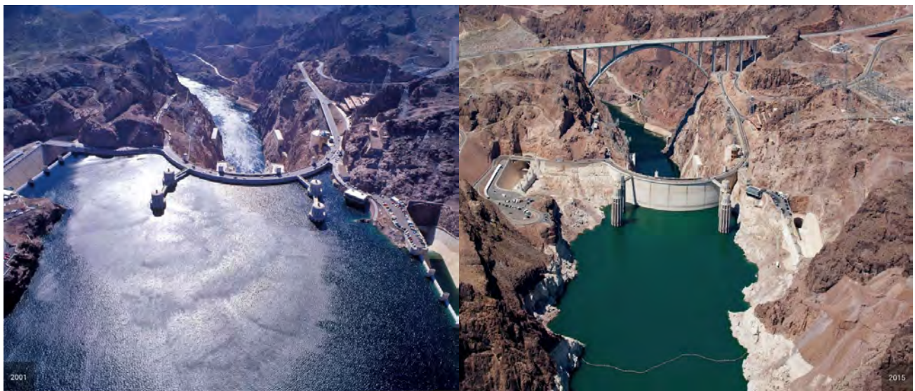
FIGURE 5 – IMPACT OF DROUGHT CONDITIONS ON LAKE MEAD. BETWEEN 2001 (LEFT) AND 2015 (RIGHT) THE LAKE ELEVATION DROPPED FROM 1,196 TO 1,075 FEET, A DECLINE OF 121 FEET. LONG-TERM IMPACTS OF EXTENDED DROUGHT CONDITIONS ON COLORADO RIVER RELIANT SYSTEMS ARE UNCERTAIN. (PHOTO CREDIT: US DOI)
